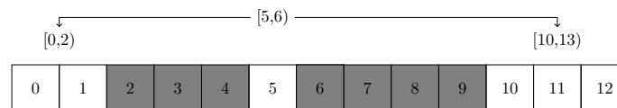
Figure 7: A fragmented pool with freeSetByIndex showing how free regions are organized in a tree structure. Index pairs are sorted left to right by the indices of the free region they represent in increasing order.
