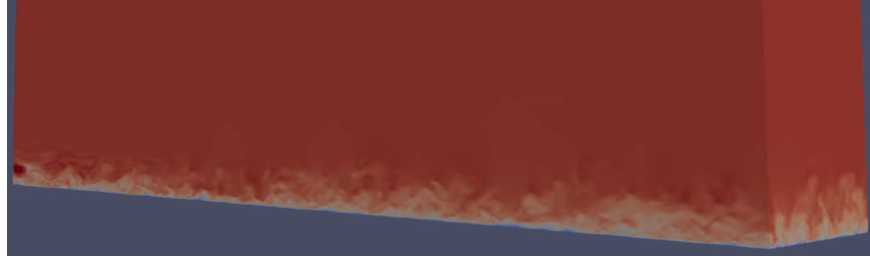
Figure 16: Velocity structure for Ma = 0.1 flat plate with STG inflow, freestream top, and the new outflow boundary condition, with the boundary layer developing from Re_\theta = 970 to 1500.
