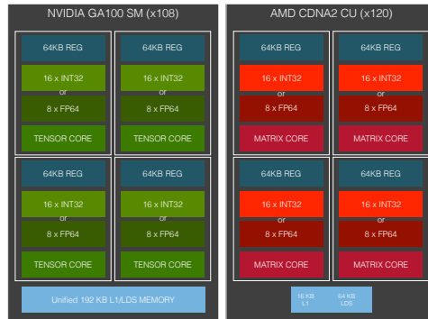
Figure 11: Comparison of the NVIDIA GA100 streaming multiprocessor and AMD MI200 series CDNA2 core architectures.
