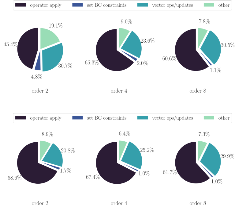
Figure 24: Breakdown of average GPU time per iteration of CG for the diffusion problem with the cuda-gen backend, on a mesh of: (top) 16 \times 16 \times 16 and (bottom) 32 \times 32 \times 32 hexahedral elements. Results obtained on an NVIDIA V100 GPU with CUDA 11.0.
